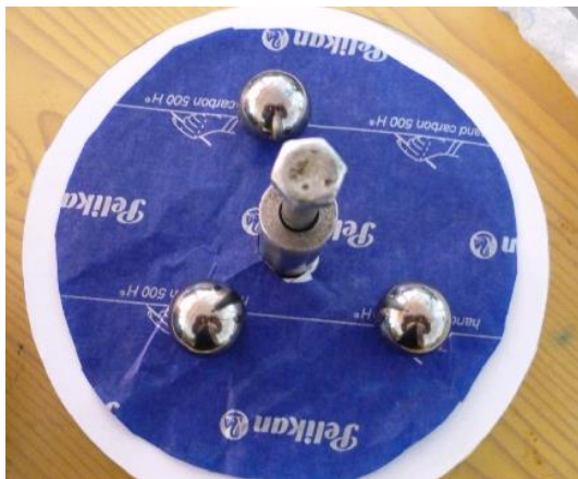
Figure 3 Immobile disc with indigo paper and three identical bearing balls on top
